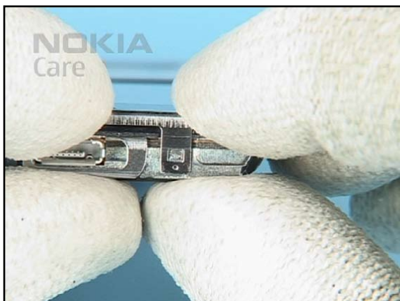
27. Close the clip on top of the unit.
