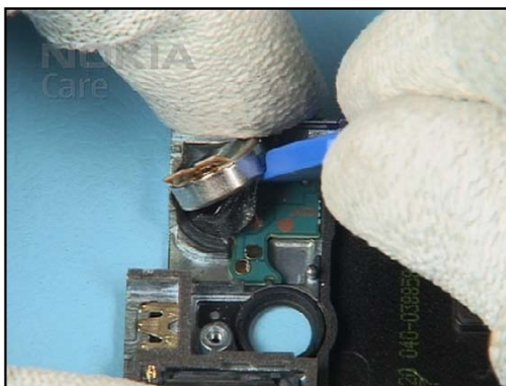
32. Remove the VIBRA and ensure that no adhesive remains.
