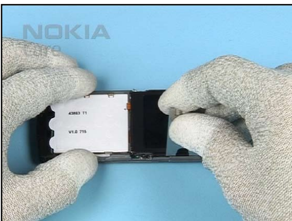
11. Release the LCD FRAME with the SS-42.
