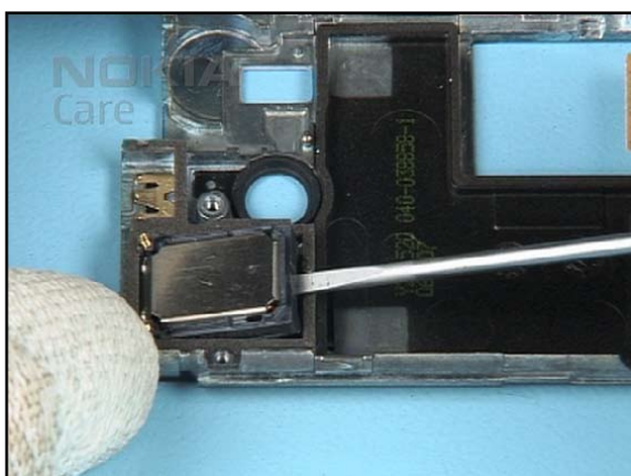
35. Carefully remove the IHF SPEAKER.
