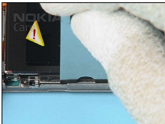
12. Place the SS-42 between the LCD FRAME and the C-COVER. Gently lever out the LCD FRAME.
