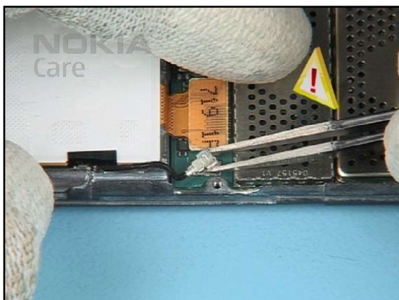
25. Carefully open the coax connector with tweezers.
