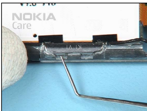
29. Unlock and remove the COAX CLAMP.
