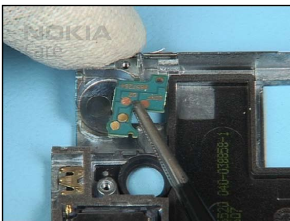
34. Discard the FLASH BOARD ASSEMBLY and also ensure that no adhesive remains.
