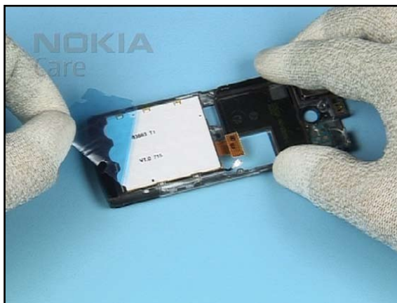
8. Remove the protection film from the UI FLEX.
