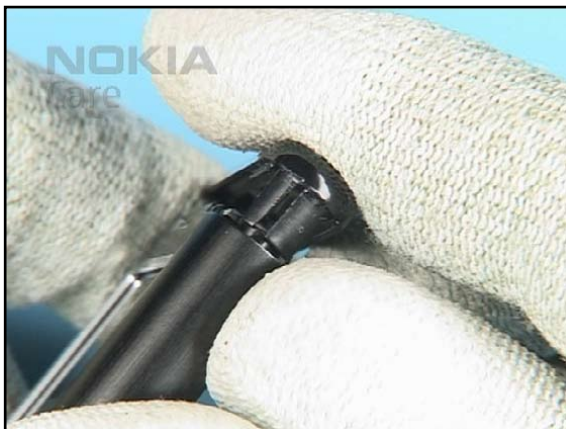
34. Always use a new TOP COVER ASSEMBLY. Pay attention to the correct position of the TOP COVER...
