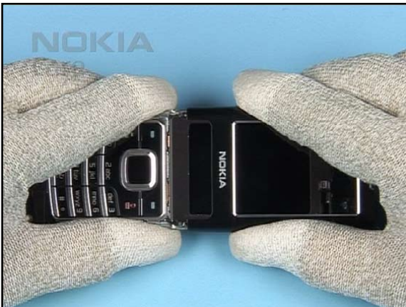
9. Carefully pull out the A-COVER.
