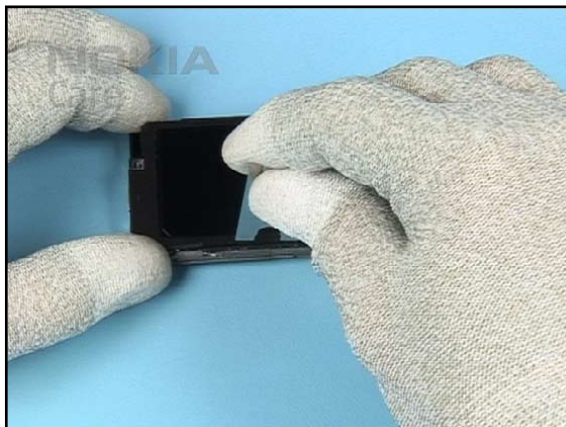
14. Now, continue on the other side of the LCD FRAME.
